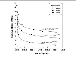
Fig. 4: Experimental S-N curves for E-glass mat chopped fiber composite plates at different layers.
